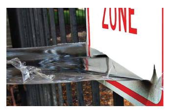
that can be applied to nearly any non-porous surface to provide a protective barrier against graffiti. After it's applied, it dries to a clear film, which protects against spray paint, marker, pen and other substances. Once defaced, the barrier is easily removed with no damage to the surface. The thickened formula adheres to vertical surfaces, and is water-resistant. allowing for some
